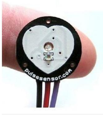
Gambar 2. 1 Sensor denyut jantung pulse sensor [5].
